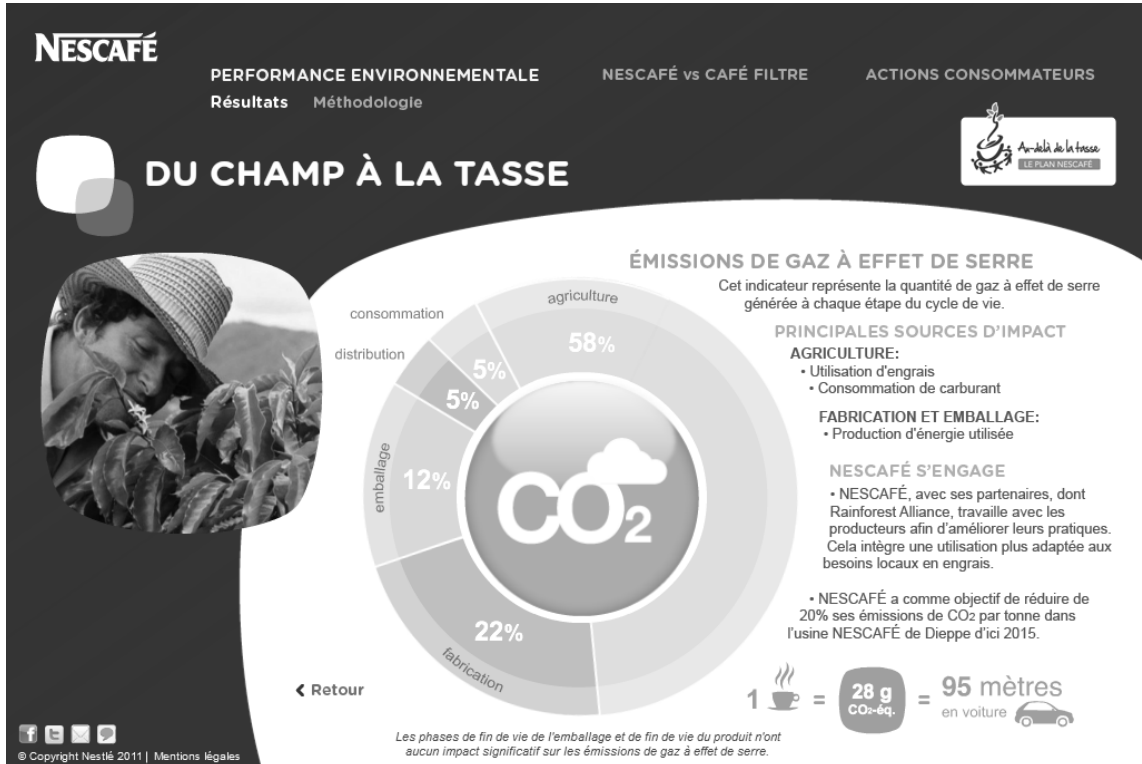
Figure 2. Nescafé® LCA Communication Tool, LCA results for the greenhouse gas emissions indicator.
